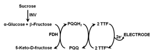
Scheme 2. Scheme showing the enzyme and electrochemical reactions involved in the sucrose determination with a INV/FDH biosensor.
